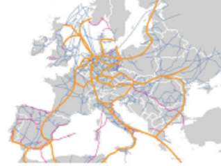
Figure 7 European Transnational hydrogen backbone - The natural gas infrastructure in Europe (blue and red lines) is suitable for a hydrogen backbone infrastructure (orange lines). The main part of the hydrogen backbone infrastructure consists of re-used natural gas transport pipelines with new compressors. At least "hydrogen transportable" must be selected from both the north and the south of the Black Sea, also along the South Coast of the Iberian Peninsula a dedicated hydrogen pipeline has to be installed.
